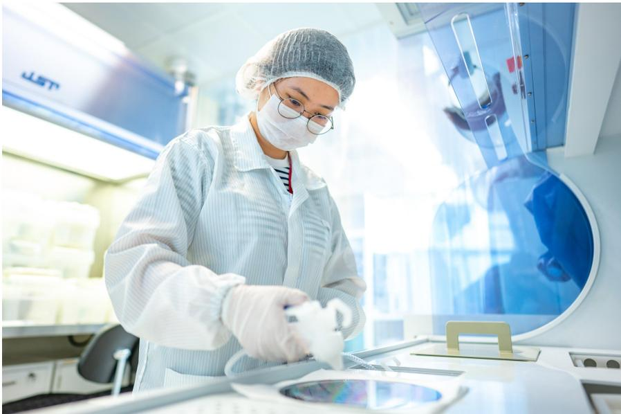
*LEES researcher reviewing a 200 mm Silicon III-V wafer. The innovative and commercial-ready process by LEES leverages existing 200 mm semiconductor manufacturing infrastructure to create a new generation of chips that combines traditional Silicon with III-V devices, something not commercially viable before.*
